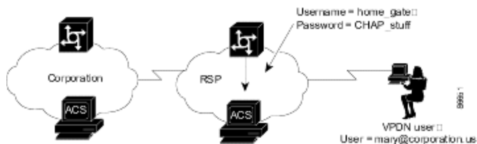
Figure D-7 NAS Authenticates Tunnel with ACS
